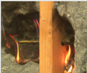
Actual wall fire in test lab caused by an Outlet AFCI failing to trip a standard circuit breaker to close the circuit in a UL1699 test
